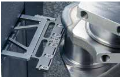
Flat measuring follower for crank shafts and convex cam shafts
