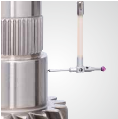
Measurement of roughness and form with double-tipped probing system and magnetic coupling
