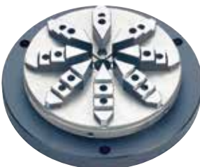
Chuck FX150 For 250 mm rotary table Chuck range Internal 46–140 mm External 2–140 mm Art. 232 359
