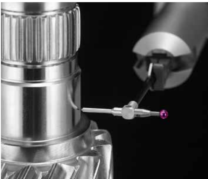
Twist measurement with a roughness stylus tip
