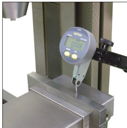
Checking the alignment on milling machine.
